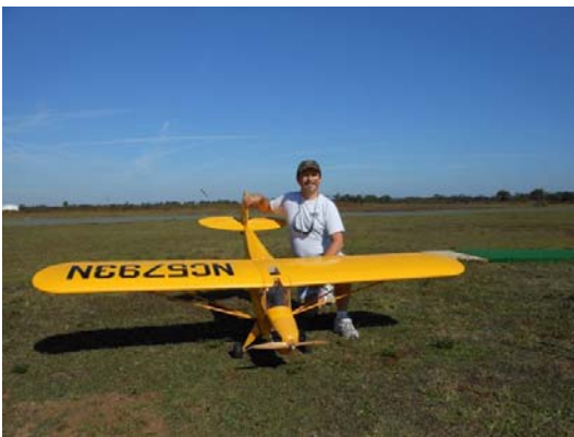
Chris Hallinan's \frac{1}{4} scale J-3 Cub features functional scale landing gear, a Saito 125, and flies like the real thing.
